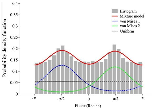
**Fig. 2.** Fitting a mixture model to circular bimodal data. The data (a gray histogram) is phase responses of the example complex RF. The red curve represents a mixture model fitted to the data according to the EM algorithm developed in Methods. This mixture model is composed of a uniform distribution (black dotted line) and two von Mises distributions (green and blue dotted lines) with different location and concentration parameters.
